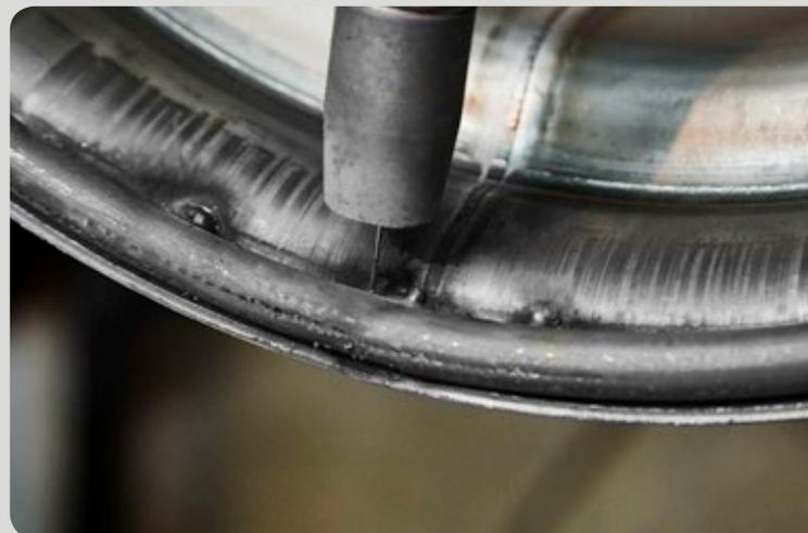
*Welding of horn reinforcement*
